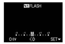
After setting, the original viewfinder/monitor screen appears again with an indication of the activated function and the compensation value
