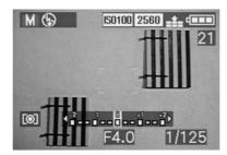
If necessary, align the shutter speed and/or aperture on the basis of the light balance and/or the histogram (see p. 138) to the desired exposure. 5. Press the shutter release button all the way down to take the photograph.
