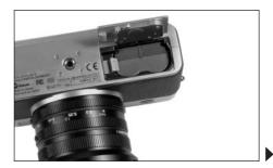
4. Close the battery compartment cover and turn the locking lever to the left.
