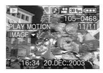
To start playback of the video recording, press down on the direction pad. You can use the direction pad as described below at any time during playback.
