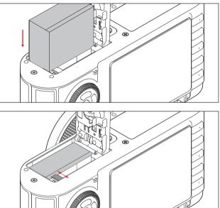
To remove the battery, follow these instructions in reverse order. The light grey sprung locking catch at the battery compartment must be pushed aside to unlock the battery.
