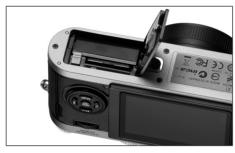
To remove the memory card, follow these instructions in reverse order. For unlocking, the card – as specified in the cover – it must first of all be pushed a little further down.
