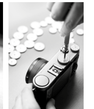
Leica X camera: fitting the shutter speed dial.
