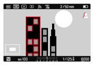
The larger the details of the object are shown, the better you can assess their sharpness and the more accurately you can focus. When Spot Metering is in use, the position of the cropped section is dictated by the position of the metering field. In all other exposure metering methods, the position is represented by cross hairs. Both can be moved to the desired position beforehand using touch control or the directional pad.
