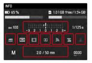
In addition to providing an overview of the most important settings, the status screen also allows quick access to specific menu functions.
