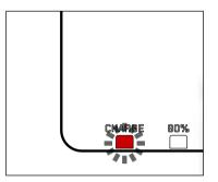
The status LED indicates a correct charging process.
