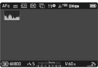
3" TFT LCD, 1.04 MP, touch control All settings are indicated in the monitor
