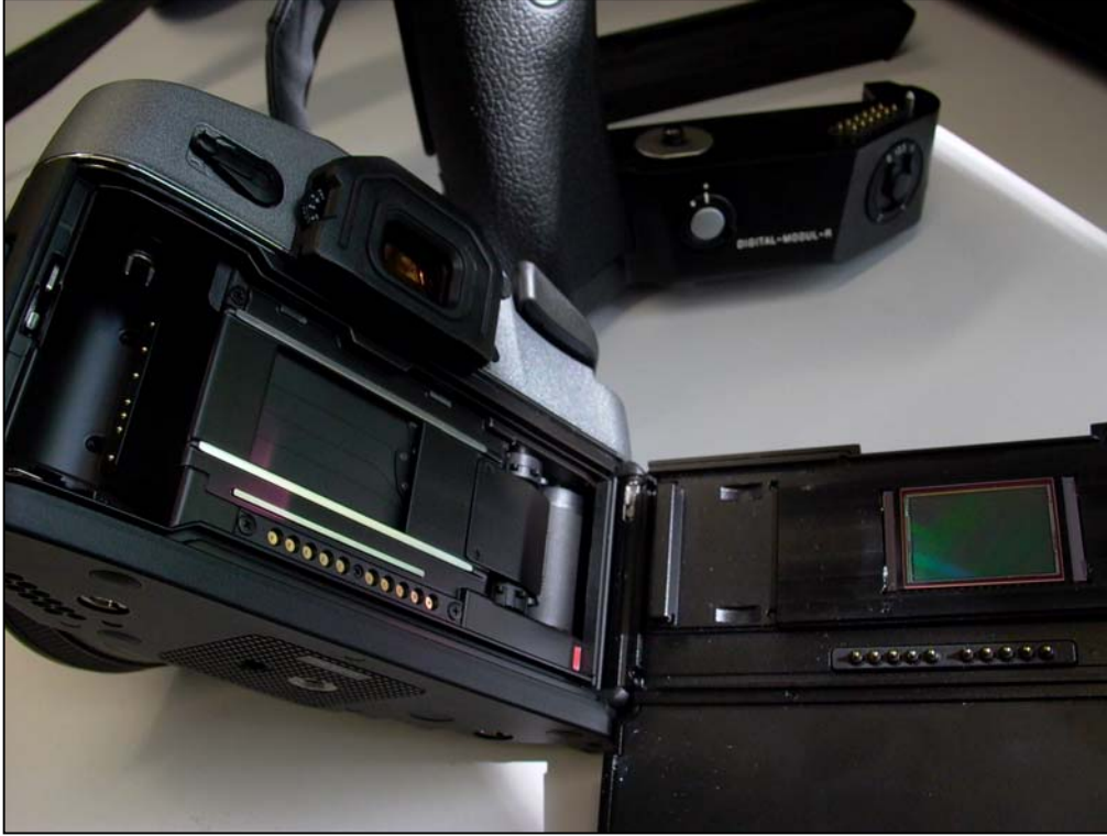
Opened Digital Back with view of sensor, power unit in background
