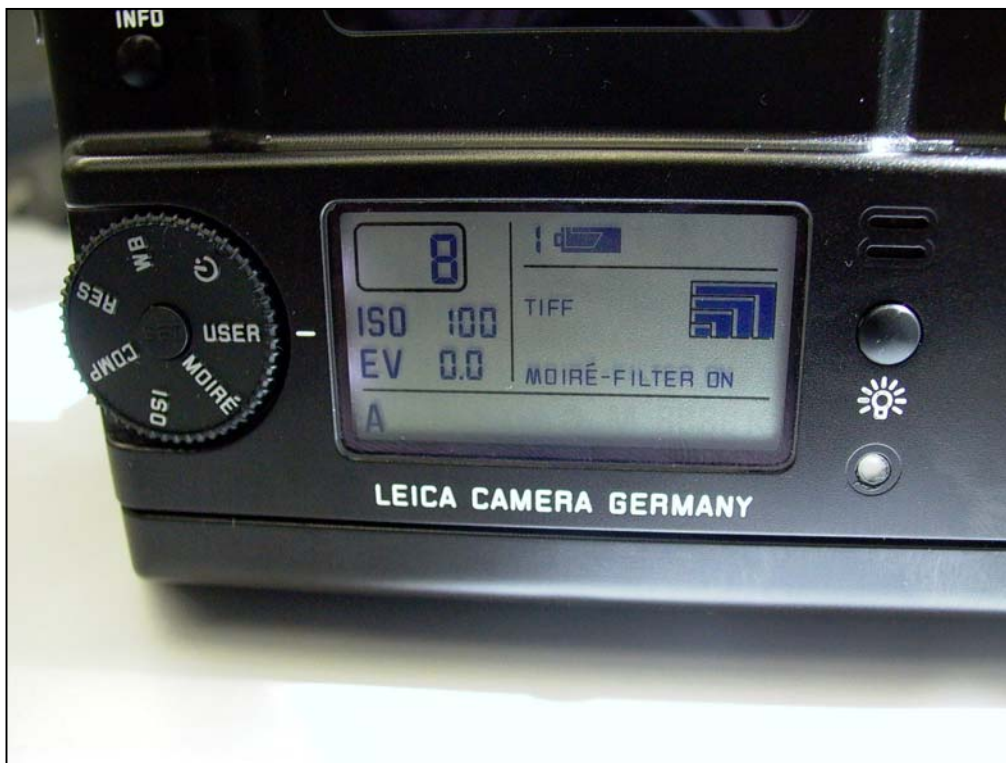
Large lighted LC display with multifunctional setting element
